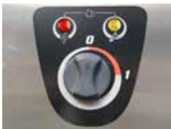
Control panel with On/off rotary switch, Led micro-leaks detector and Alert ordinary pump maintenance device
